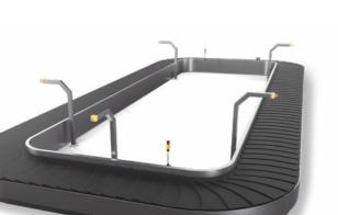
sections, allowing to create the desired shape of the carousel. The carousel is equipped with a friction drive, which enables very silent operation. Specially cast chain – very light and durable, ensures trouble-free operation. Thick slats are available in various colours. The inclined configuration of the carousel guarantees better ergonomics of use which facilitates quick and simple baggage claim.
